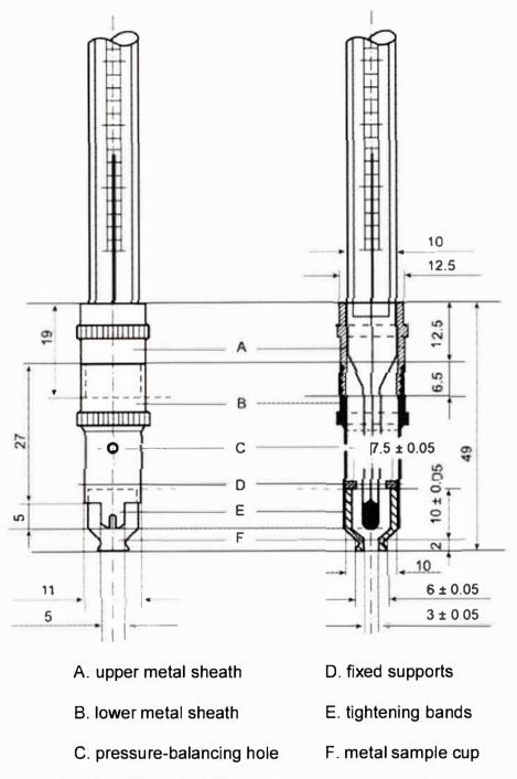
Figure 1. Apparatus for the determination of drop point Dimensions in millimeters
