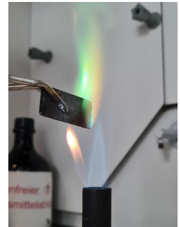
Beilstein test positive
